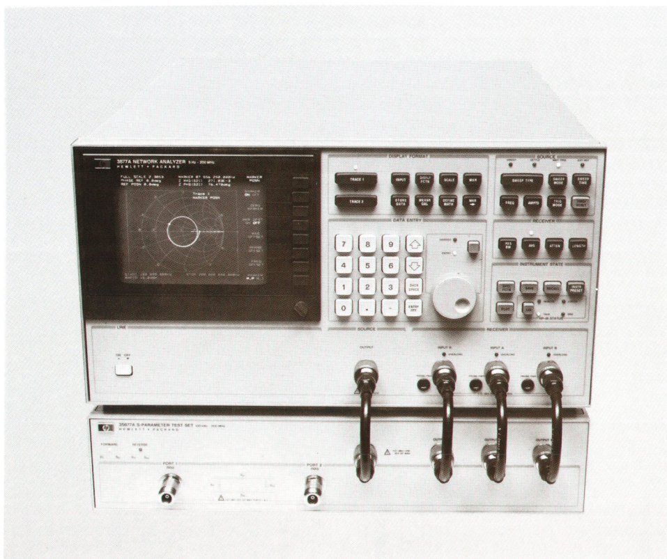
Fig. 1. The HP 3577A Network Analyzer (top) provides cost-effective, high-performance network measurements. The companion HP 35677A/B S-Parameter Test Set (underneath) and a full line of accessories ensure a comprehensive measurement solution. Convenient softkey selection of measurement functions allows the user to measure transfer functions, magnitude/phase, insertion loss/gain, attenuation, electrical length, group delay, and gain compression.
