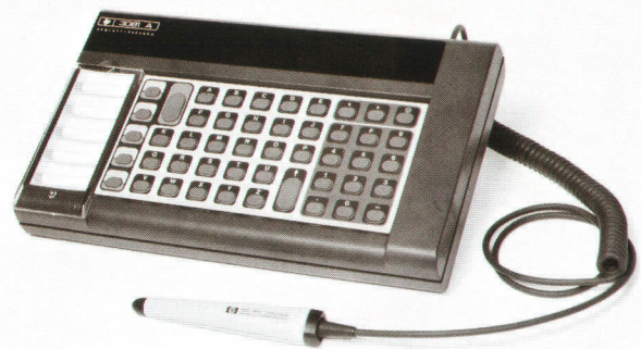
Fig. 2. Options include an alphanumeric keypad, a choice of bar code wands, and a choice of slot readers.
